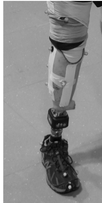
Figure 35: Prosthesis with iPecs sensor below the socket
